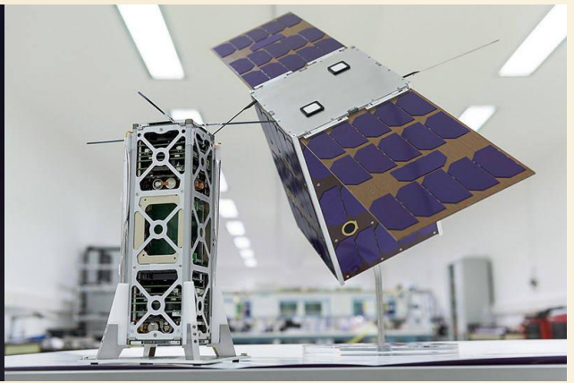
View of the first Argos Nanosatellite ANGELS (on the right), precursor of the future Kinéis nanosat, with an Argos-4 payload. The constellation of 20 nanosats makes it possible to have a much faster revisit time.
