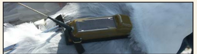
Gull with 17g GPS transmitter. Closeup of transmitter on gull.
