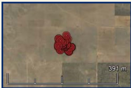
A customer was concerned that one of his GPS transmitters might be down (due to bird mortality or transmitter detachment) as the temperature and battery voltage had dropped for several days. A quick look at a graph of latitude and longitude data showed us that the locations were changing by distances greater than the margin of error for GPS; from this we could conclude the animal was still active.
