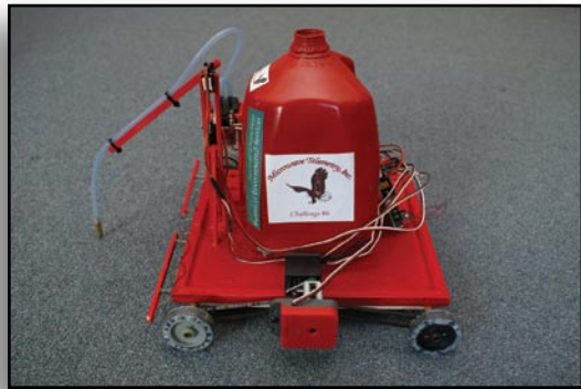
Red the Robot: the winning entry of Challenge 06. Red weighed 2.25 lbs., carried one gallon of water, and had an ingenious design incorporating optical encoders around the wheels and bumper switches at the front.
