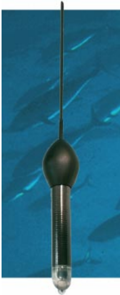
Archival Pop-up tags record the water temperature and depth as well as the time of sunrise and sunset each day. These times are transmitted back to the user via Argos after the tag pops up. They are subsequently used to calculate a daily location estimate and hence reconstruct the track of the fish.
