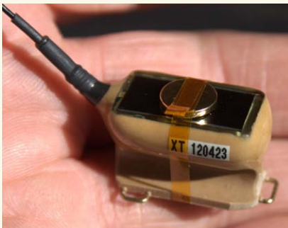
A solar-powered PTT with lift-kit base. Total weight of modified unit with Teflon tubing harness is 6.2 g. The shape minimizes aerodynamic drag and weight, and allows the owls' feathers to be groomed alongside the unit.
